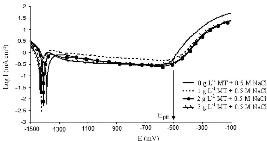
FIGURE 2. The potentiodynamic polarisation curves of Al alloy containing various concentration of MT in 0.5 M NaCl at pH 12
