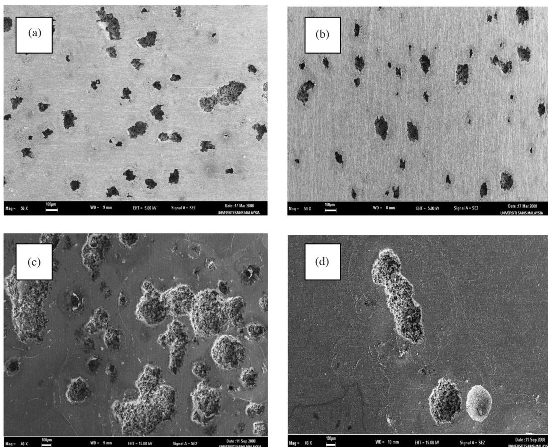
FIGURE 3. SEM micrograph of Al alloys in (a) 0.5 M NaCl pH 6 (b) 0.5 M NaCl pH 6 + 3 g L<sup>-1</sup> MT (c) 0.5 M NaCl pH 12 and (d) 0.5 M NaCl pH 12 + 3 g L<sup>-1</sup> MT
